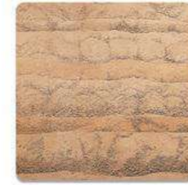
AYB7 rammed earth (soft)
