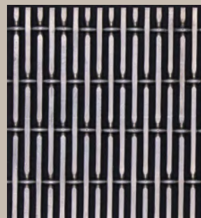
QKCWM-10 Warp Diameter:1.5mm Weft Diameter:2mm Warp Pitch:4mm Weft Pitch:17.5mm Weight:2.5kg/m 2 Opening Area:45.7%
