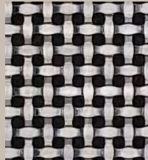
QKCWM-07 Warp Diameter:0.75x2mm Weft Diameter:0.75x2mm Warp Pitch:15mm Weft Pitch:15mm Weight:6.5kg/m 2 Opening Area:9.2%
