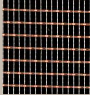
QKCWM-16 Warp Diameter:0.8mm Weft Diameter:1.5mm Warp Pitch:2.88mm Weft Pitch:7.25mm Weight:4.1kg/m 2 Opening Area:53.9%
