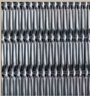
QKCWM-22 Warp Diameter:2mm Weft Diameter:1.5mm Warp Pitch:17.5mm Weft Pitch:1.55mm Weight:11.67kg/m 2 Opening Area:0%
