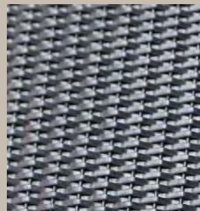
QKCWM-23 Warp Diameter:2.5mmx3 Weft Diameter:3mm Warp Pitch:90.5mm Weft Pitch:12mm Weight:6.08kg/m 2 Opening Area:68.8%
