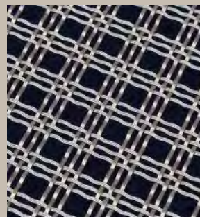
QKCWM-14 Warp Diameter:1.2x3.5mm Weft Diameter:1.2x3.5mm Warp Pitch:42mm Weft Pitch:42mm Weight:4.8kg/m 2 Opening Area:58.7%
